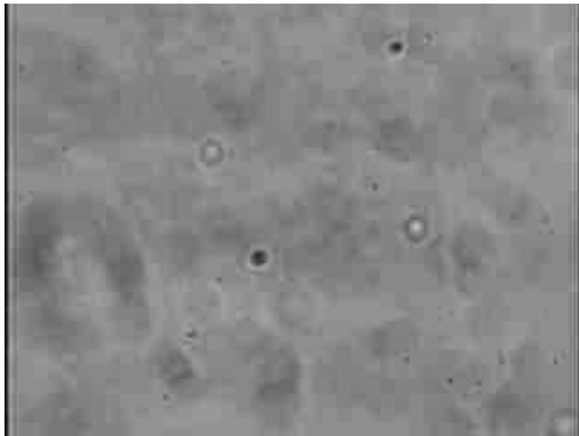
Trapped polystyrene bead using two CARS beams
